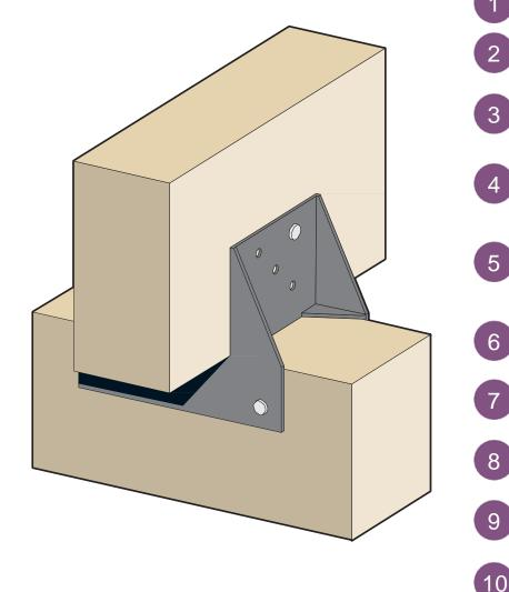
Provides a positive connection between joist and bearer.
